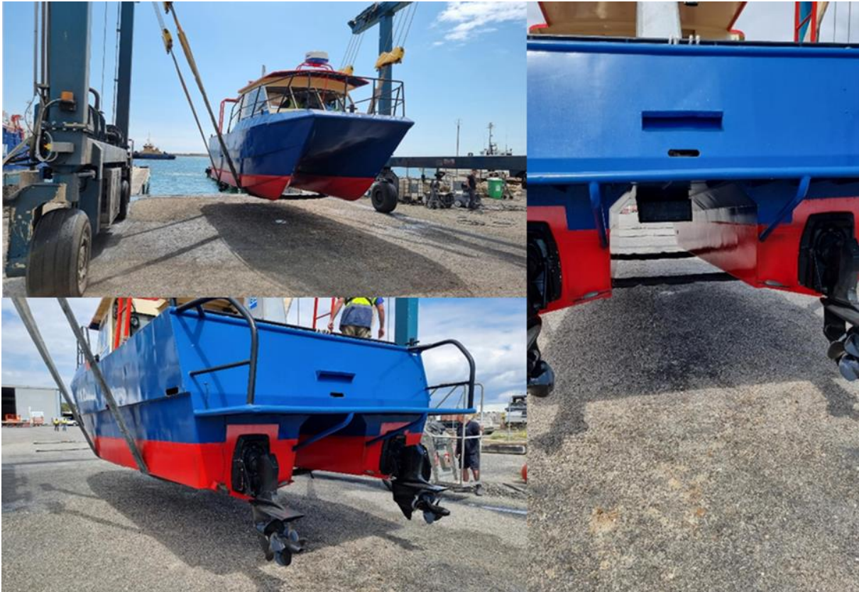
Figure 2.27 Images of the hull of hydrographic survey vessel Rind-R showing newly applied anti-foulant coating prior to launch at Carnarvon, Western Australia
