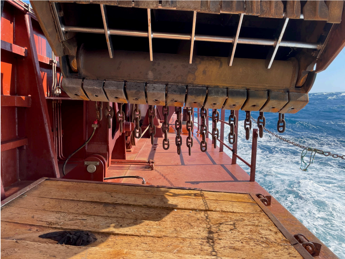
Figure 5: Photograph of the “Sea Turtle Deflector” attached to Modi R draghead
