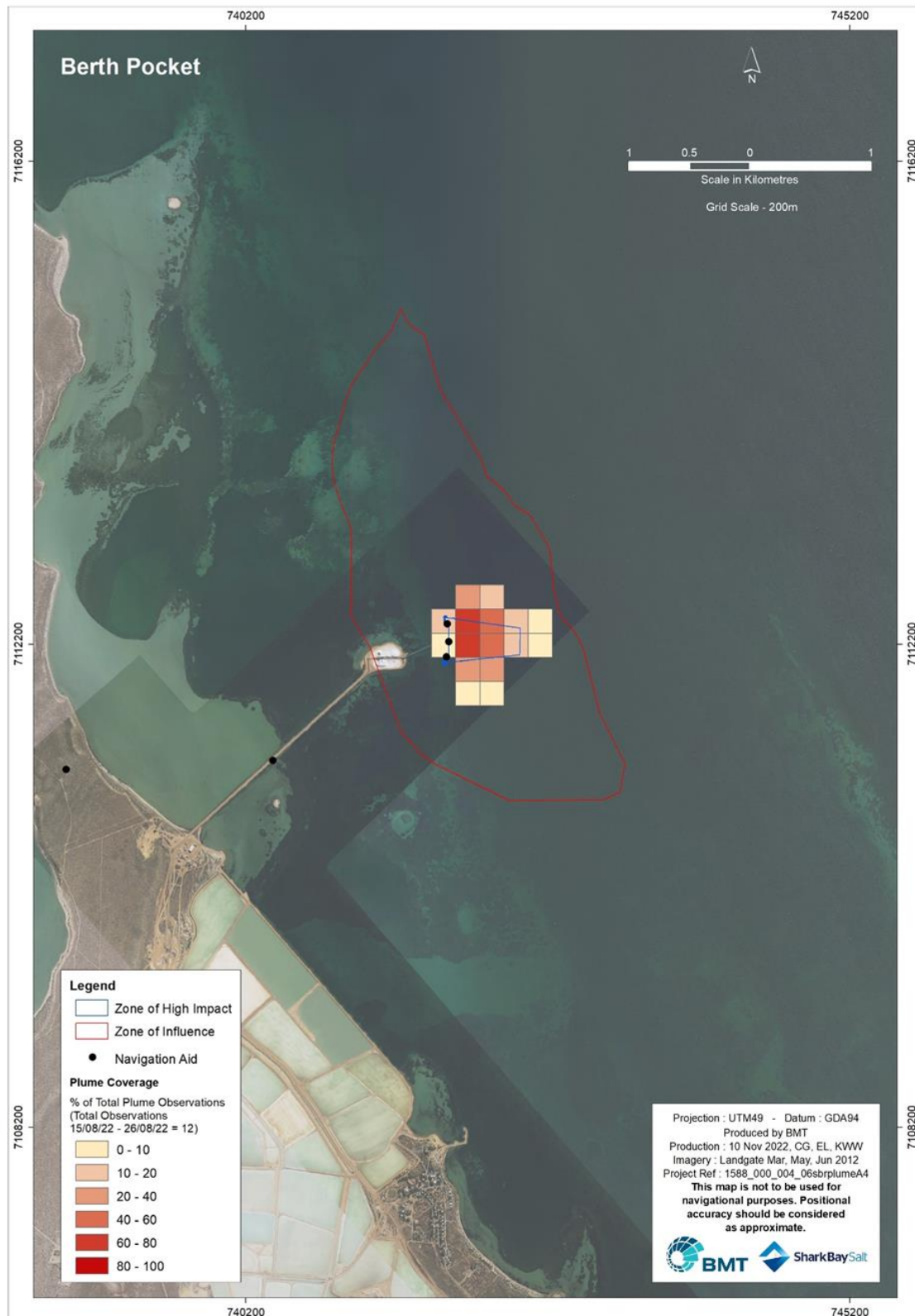
Figure 2.4 Plume coverage map of the seabed levelling operations in the Berth Pocket during the Useless Loop maintenance dredging campaign
